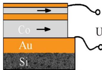
*Schematic image of the functional element of the magnetic field sensor based on the spin-valve*
